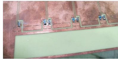
PCB strip panel for BIS78
