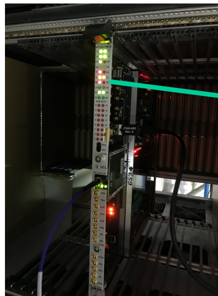
TIM (@VME-3) showing fiber input from the LHC
