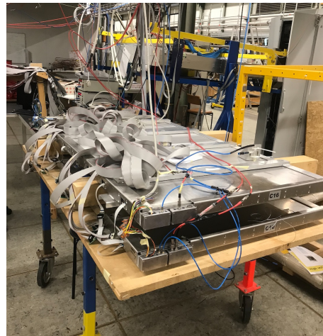
Preparing setup (RPC singlet + doublet) for efficiency measurement after integration @BB5
