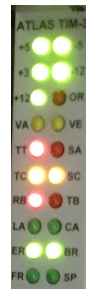
LEDs lighting up (ER, BR) after fiber input from LHC/ATLAS
