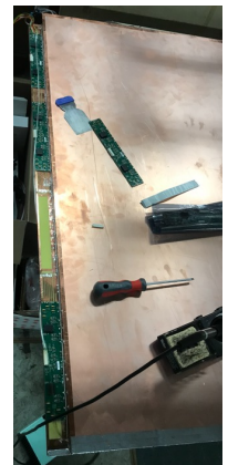
Replacing FE board/s to fix dead channels
